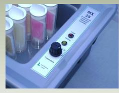
Temperature & status indicators are safe from knocks under the lid, a  $\underline{37}^{0}\underline{c}$ <u>Quickset</u> point helps easy initial set up
